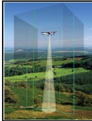
Fixed wing based laser systems for Liq/N-Gas vapor detection
