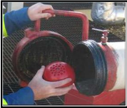
Internal Liq/N-Gas LDS transferred from the water pipeline industry
